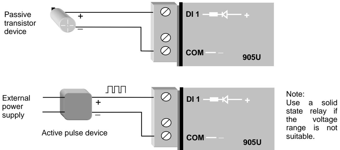
Active pulse signals can be connected directly provided the peak voltage is between 3.5–13V and the low voltage is less than 1.5V. Note that the 905U will ground the negative of the pulse signal. If the voltages are not compatible, use a solid state relay to isolate the two devices.
