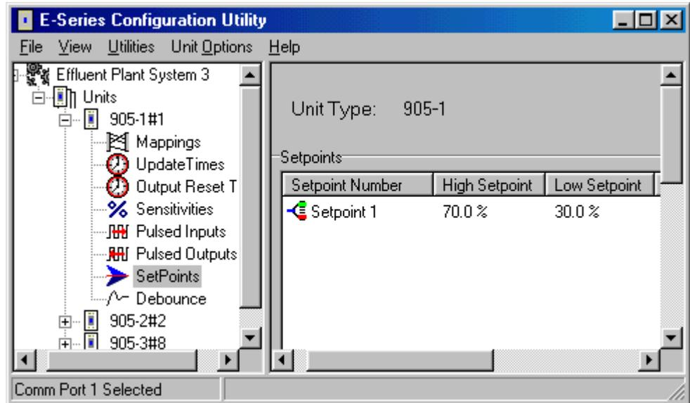
Set Point (HSP) must always be higher than the Low Set Point (LSP). For the -1 module, only AI1 has set-point values. For -2 modules, the first four analog inputs (AI 1 – 4) have set-points.
