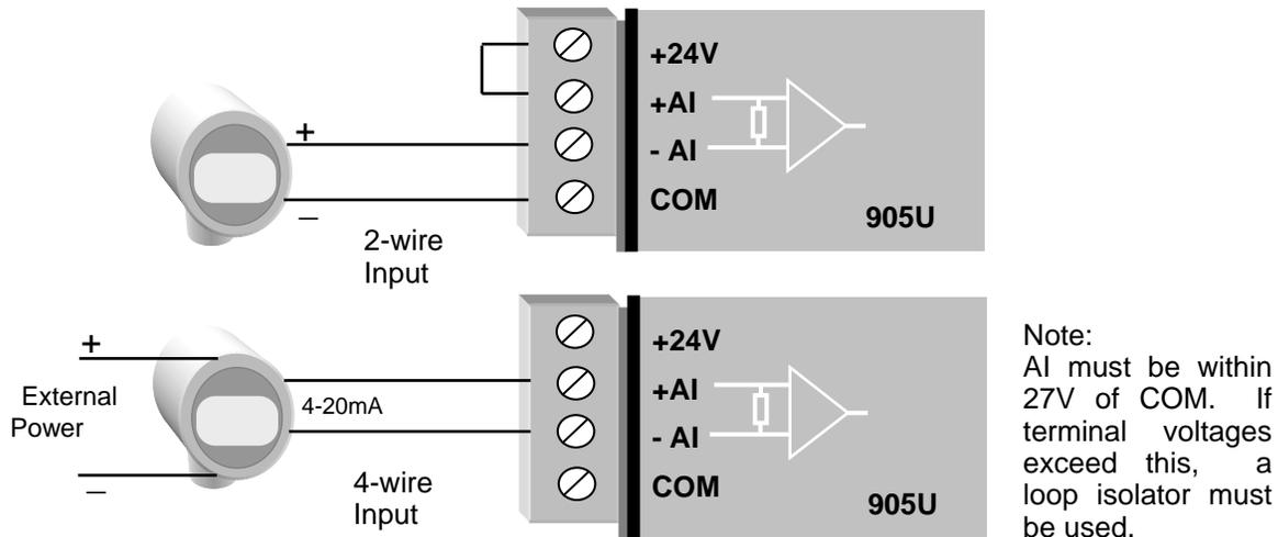
Externally powered loops may be connected by connecting the input between "AI 1+" and "AI 1-" for analog input 1 or "AI 2+" and "AI 2-" for analog input 2, and so on for other inputs. Common mode voltage may be -0.5V to 27V.
