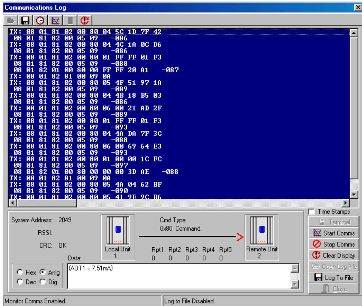
If you select any message line with the mouse, information about the message will be displayed at the bottom of the screen - the system address, RSSI and CRC (error-check) status. The “text box” at the bottom middle of the screen decodes the message - that is, it decodes the message to display I/O channel and value.
