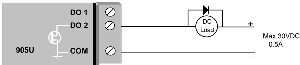
Digital outputs may be configured to individually turn off if no command message is received to that output for a certain period. This feature provides an intelligent watch dog for each output, so that a communications failure at a transmitting site causes the output to revert to a known state. See Chapter 4 Configuration for further details.
