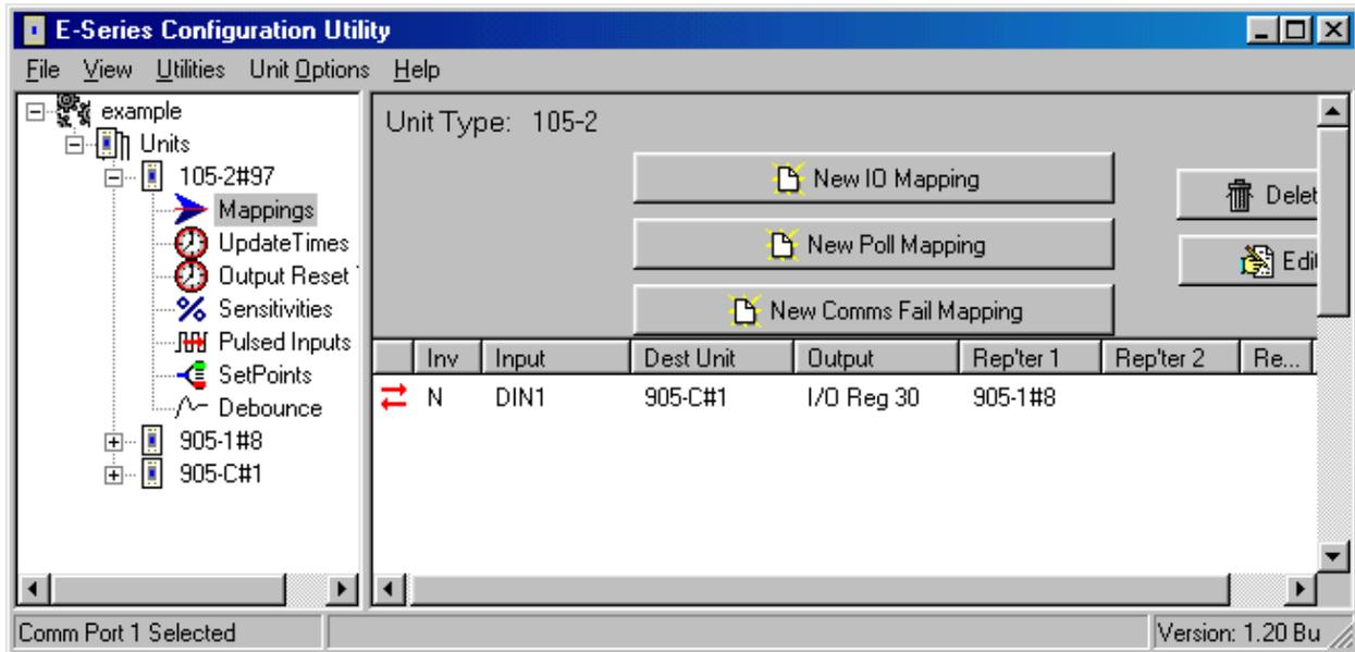
In this example, a 105S-2 is connected to 905U-1#8. DI1 is mapped to a remote 905U-C module. The 905U that is connected to the 105S module acts as a repeater - a serial-to-radio repeater.
