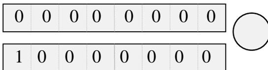
Input signals may now be connected to the input terminals of the module. If the module is operating correctly, then the input signals will be reflected to the corresponding output on the same module. For example, if DI 1 is connected to common - i.e. the first digital input is turned "ON" - then DO 1 will activate, if the module is functional. Similarly, if a 12mA signal is connected to AI 2, then a 12mA signal should be able to be measured from AO 2, if the module is functioning correctly.
