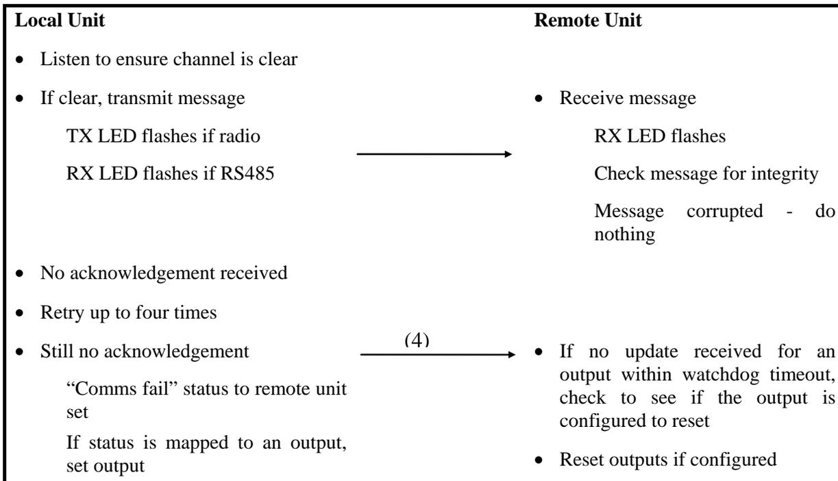
If communications is still not successful, the “Comms Fail” internal status will be set. In the default configuration, this will have no consequence and the module will continue to attempt to transmit to the remote module every ten minutes. For critical applications, the “comms fail” status can be configured
