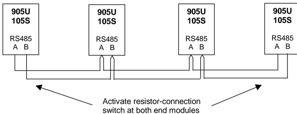
105S modules connect to a 905U via the RS485 port on each module - refer to section 2.4.11. Up to 31 x 105S modules can be connected to a 905U module. This number is reduced for 105S-3 and -4 modules, as these modules use two unit addresses (refer to chapter 4 of this manual).
