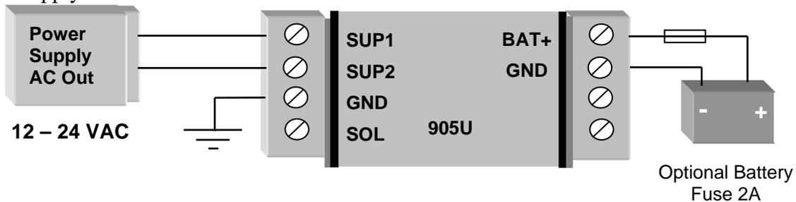
The AC supply should be "floating" relative to earth. AC transformers with grounded/earthed secondary windings should **not** be used.
