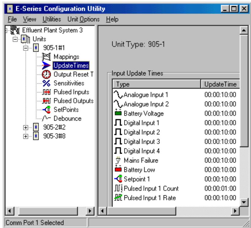
each field. The display also shows the maximum and minimum values. For the -1, -2 and -3 modules, the maximum update time is 16 minutes, however the update time for -4 inputs can be up to 5 days.
