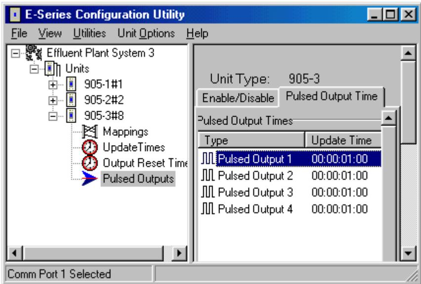
To configure the pulse output time, select “Pulse Outputs” on the left-hand menu and select the “Pulsed Output Time” page - double-click the pulse output and enter the new time.
