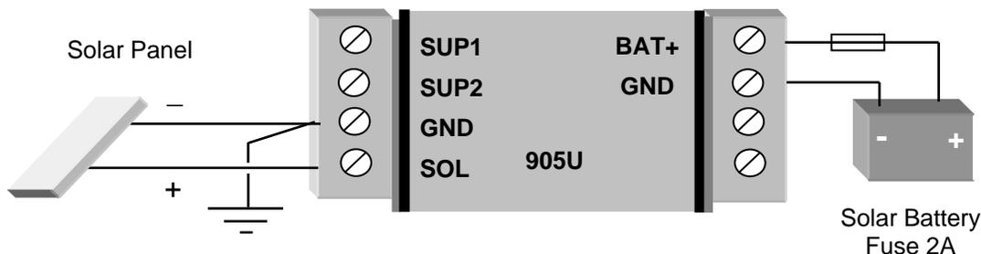
The solar panel is connected to the "SOL" (positive) and "GND" (negative) terminals and the battery connected to the "BAT+" (positive) and "GND" (negative) terminals. Solar panels must be installed and connected as per the panel manufacturer's instructions. The positive lead of the battery should be protected by a 2A fuse installed as near as possible to the battery terminal.
