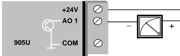
A 24VDC supply is available on the module for powering the analog output loop (max external loop resistance 1000 ohms). In this case, the analog loop is connected between a "+24V" terminal and "AO 1" (for the first analog output) or "AO 2" (for the second analog output), and so on for the other output signals.
