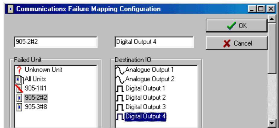
Each remote module has a separate comms fail status - you enter a separate comms fail mapping for different remote addresses. You can configure several comms fail mappings to the same output - the output will be active if there is comms fail to any of the remote addresses. Configuring a “Comms Fail Address” of zero causes communication failure to any destination module to be indicated on the selected output.
