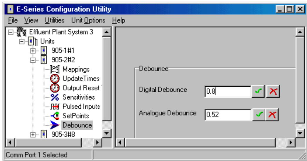
Debounce may be configured for digital inputs on the -1, -2 and -4 modules (0.5 - 8 seconds) and the analog inputs on the -2 module (0.5 - 8 seconds). The default value of 0.5 seconds is suitable for most applications. In applications where a digital input may turn on and off several times slowly (for example, security switches or float switches) a debounce time of up to 8 seconds may be configured. *The configured debounce time has no affect on pulse inputs.*
