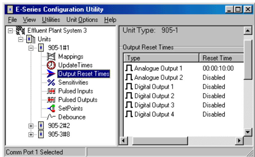
If the reset time is less than the update time, then the output will reset when the reset time expires, and then set again when the update message is received. We recommend that the reset time be a little more than twice the update time.
