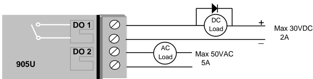
Digital outputs may be configured to individually turn off if no command message is received to that output for a certain period. This feature provides an intelligent watch dog for each output, so that a communications failure at a transmitting site causes the output to revert to a known state. See section 4.4 Changing User Options for further details.
