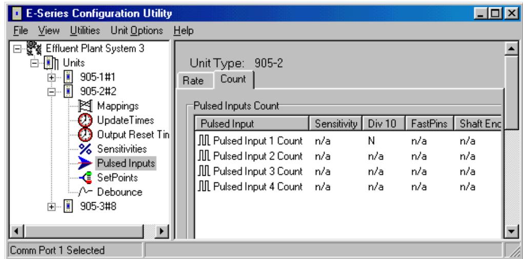
To configure the “divide by 10” feature, select “Pulse Inputs” on the left-hand menu and select the “Count” page - double-click “Pulse Input 1 Count” and enable “divide by 10” counting.
