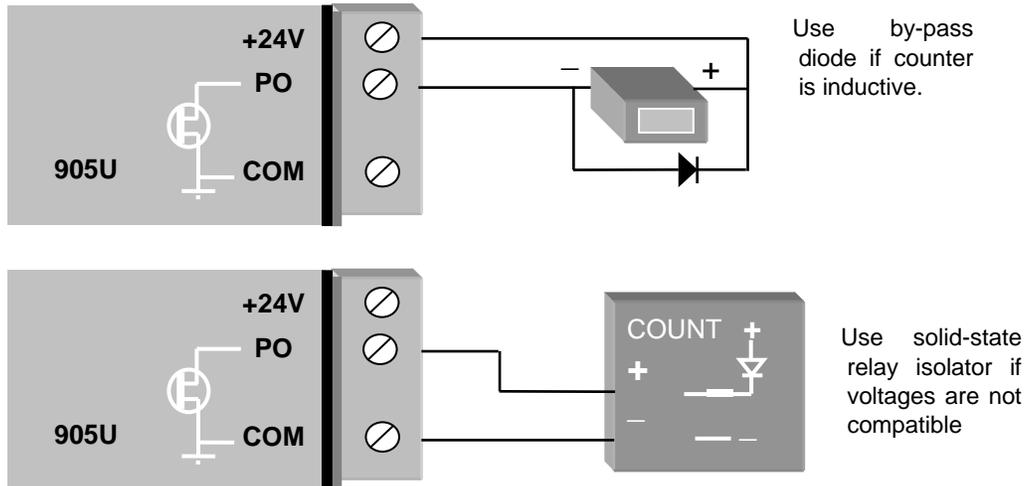
If the counter device requires a voltage pulse signal (such as electronic or elector-mechanical counters), use the 24V analog loop supply, or the 12V BAT supply for the voltage source. Use a by-pass diode if the counter is inductive.
