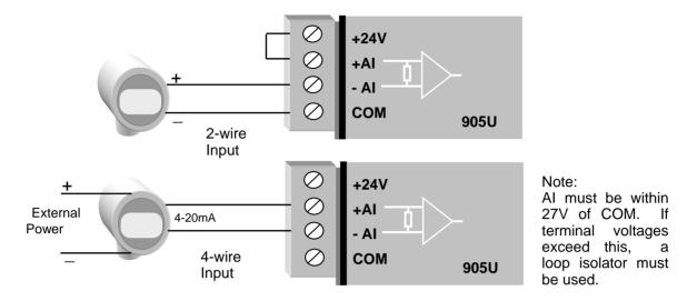
Externally powered loops may be connected by connecting the input between "AI 1+" and "AI 1-" for analog input 1 or "AI 2+" and "AI 2-" for analog input 2, and so on for other inputs. Common mode voltage may be -0.5V to 27V.
