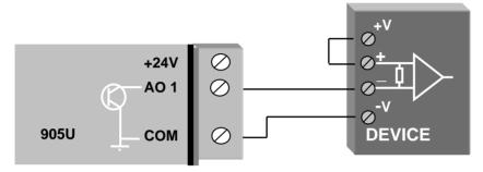
Note: COM on 905U is connected to ground/earth. If the external power supply cannot be grounded, a loop isolator must be used.
