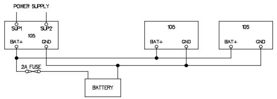
For example, assume there is a 905U-1 module and a 105S-1 module at the same location. The total I/O at the location is 3 analog inputs, 6 digital inputs and 4 digital outputs. The total load will be :-
