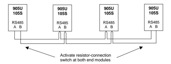
105S modules connect to a 905U via the RS485 port on each module - refer to section 2.4.11. Up to  $31 \times 105S$  modules can be connected to a 905U module. This number is reduced for 105S-3 and -4 modules, as these modules use two unit addresses (refer to chapter 4 of this manual).
