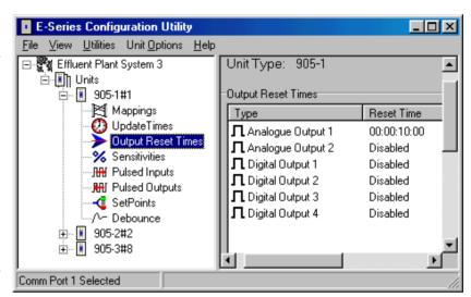
should be configured to reset on communications failure so that the pump will turn off. The default condition is zero (no reset).
