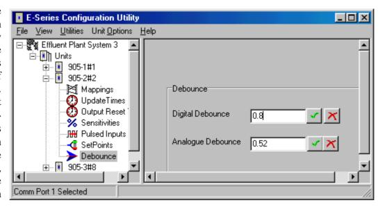
Debounce may be configured for digital inputs on the -1, -2 and -4 modules (0.5 - 8 seconds) and the analog inputs on the -2 module (0.5 - 8 seconds). The default value of 0.5 seconds is suitable for most applications. In applications where a digital input may turn on and off several times slowly (for example, security switches or float switches) a debounce time of up to 8 seconds may be configured. The configured debounce time has no affect on pulse inputs.
