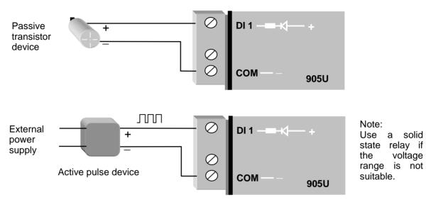
Active pulse signals can be connected directly provided the peak voltage is between 3.5–13V and the low voltage is less than 1.5V. Note that the 905U will ground the negative of the pulse signal. If the voltages are not compatible, use a solid state relay to isolate the two devices.
