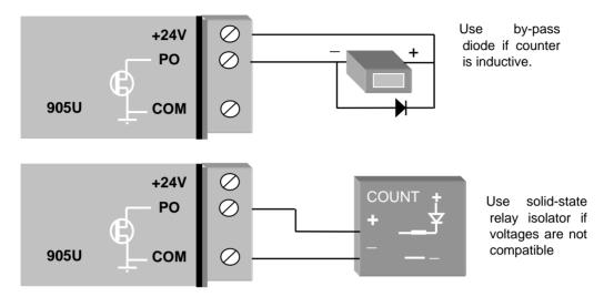
If the counter device requires a voltage pulse signal (such as electronic or elector-mechanical counters), use the 24V analog loop supply, or the 12V BAT supply for the voltage source. Use a by-pass diode if the counter is inductive.
