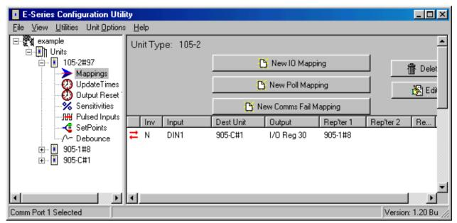
In this example, a 105S-2 is connected to 905U-1#8. DI1 is mapped to a remote 905U-C module. The 905U that is connected to the 105S module acts as a repeater - a serial-to-radio repeater.
