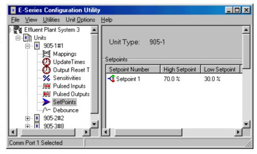
Set Point (HSP) must always be higher than the Low Set Point (LSP). For the -1 module, only AI1 has set-point values. For -2 modules, the first four analog inputs (AI 1 - 4) have set-points.
