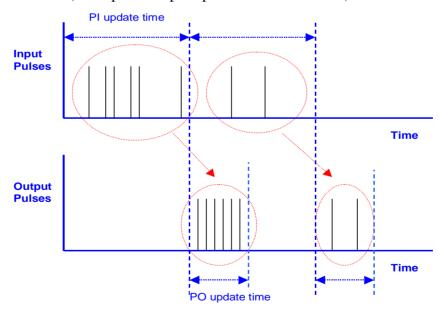
The default values for the pulse input update time and pulse output update time is 1 minute. In this case, the output pulses are effectively 1 minute behind the input pulses. These update times may be changed by the user. The pulse output update time should not be set to be more than the pulse input update time. Note that the maximum pulse rate for both inputs and outputs is 100Hz.
