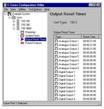
and then by the serial link to #96. If anything happened to either module #2 or module #1, or the radio link, or the serial link, then the update messages for DO4 will not be received at the control station module. After 3.5 Minutes, DO4 will reset indicating a problem.
