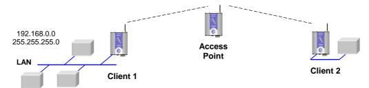
Configure units as described in Section *Extending a wired network*. Place the Access Point at the remote intermediate repeater location.
