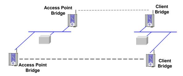
For example, consider this network with a redundant wireless link. If the Spanning Tree Algorithm function is enabled, one of the two wireless links will be disabled - that is, all wireless data will be transferred by one link only. If the active link fails, the other link will automatically start transferring the wireless data.
