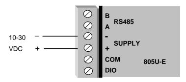
Transmission current (500mW RF) is nominally 500mA at 12V, 250mA at 24VDC.
