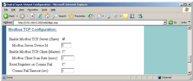
Unit C is configured with Modbus TCP Server enabled and Device ID = 1, so that the Modbus TCP Client at B can connect and read the status of the onboard digital input. Unit C also has Modbus TCP to RTU Gateway enabled (see section "3.13.3 Modbus TCP to RTU Gateway") so that the Modbus TCP Client at B can communicate with the serial Modbus RTU device D.
