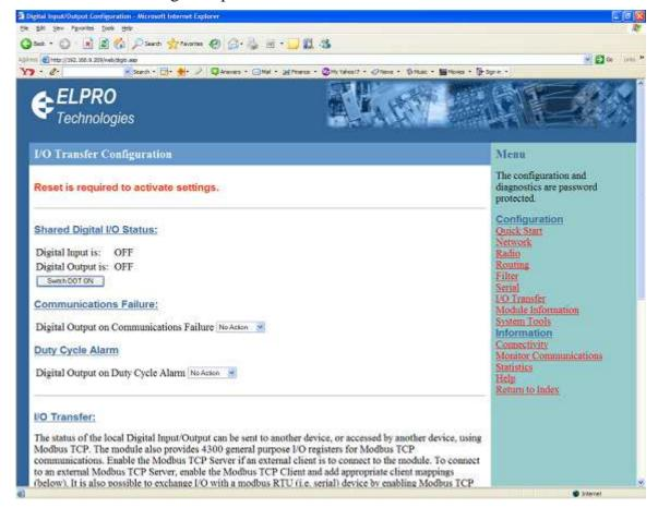
The shared Digital Input/Output pin may be monitored and set via the internal webpage. As this pin is shared, the Digital Input status will be ON when the Digital Output is set ON.
