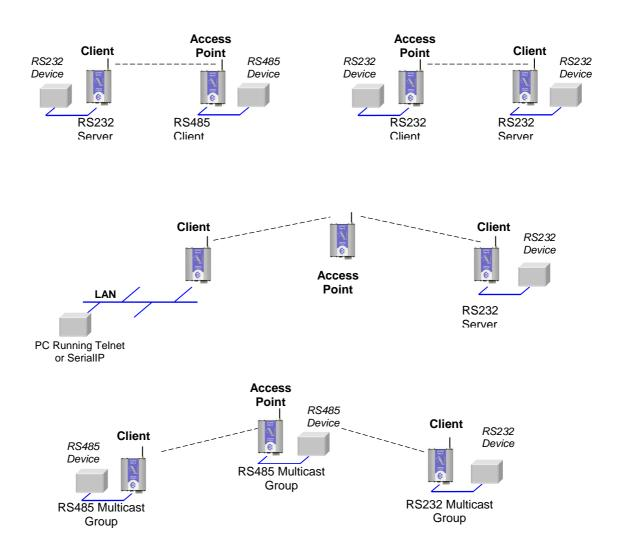
There are software packages available (i.e. SerialIP Redirector by Tactical Software) that can create a virtual serial port on a PC. This virtual serial port can be configured to connect to a 805U-E serial port. Standard programs can then be used to access this serial port as if it were actually connected to the PC. Alternatively the program telnet may be used to connect to a serial port on the 805U-E. The telnet command used should be:
