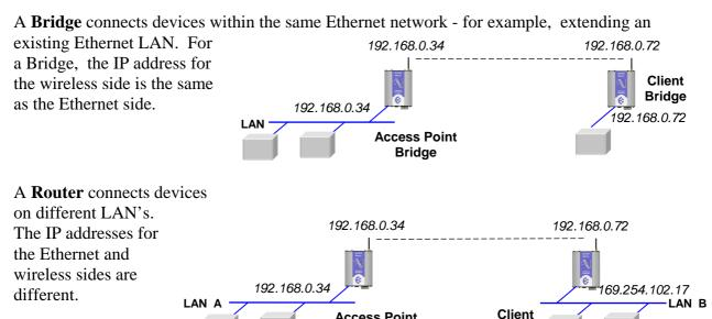
In the above example, the wireless link is part of LAN A, with the Client unit acting as a Router between LAN A and LAN B. Alternately, the Access Point could be configured as a Router the wireless link is then part of LAN B.
