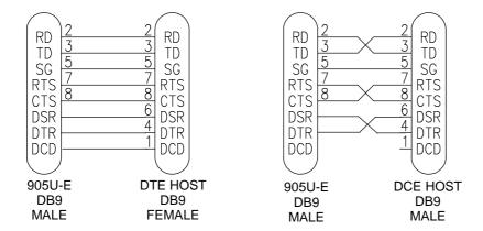
Hardware handshaking using the CTS/RTS lines is provided. The CTS/RTS lines may be used to reflect the status of the local unit's input buffer, or may be configured to reflect the status of CTS/RTS lines at the remote site. The 805U-E does not support XON/XOFF.
