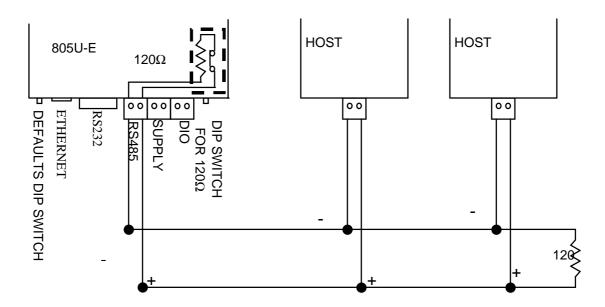
RS485 CONNECTION USING TERMINATING RESISTOR
