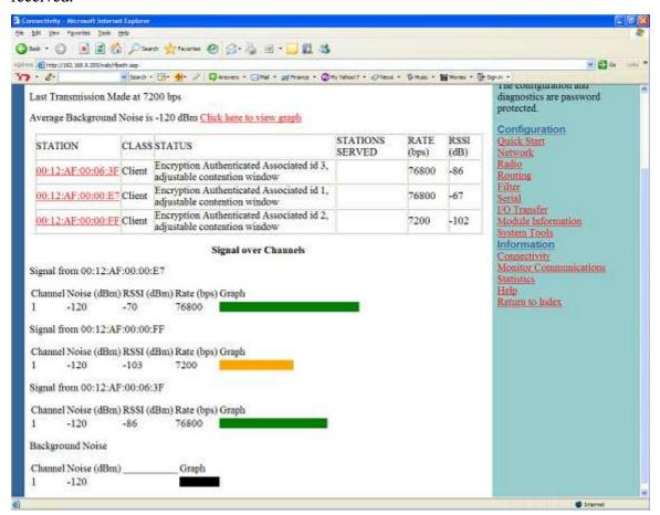
The table shows the averaged receive signal strength and last received radio data rate for each Client or Access Point by their MAC Address. The unit listed at an Access Point may not even be in the same system. This can provide an idea of how busy the radio band is.
