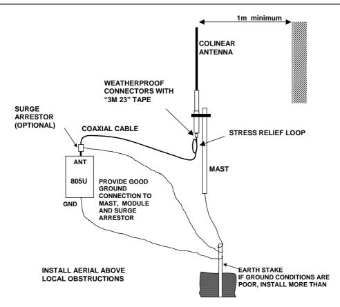
Collinear and dipole antennas should be mounted vertically, preferably 1 metre away from a wall or mast to obtain maximum range.
