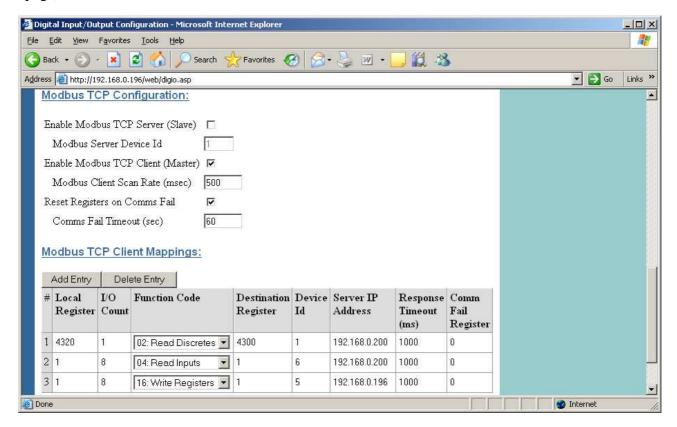
It can be seen that Modbus TCP Client has been enabled with a 500msec scan rate, meaning that there will be a 500msec delay between each of the *mappings* directed at any server. The "Reset Registers on Comms Fail" option is enabled with a timeout of 60 seconds, indicating
